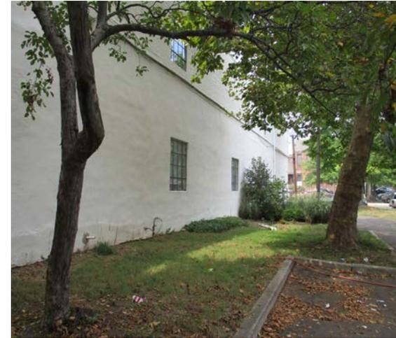
This site is the location of Isle’s Tucker Street office and community garden. Roof runoff currently drains directly to the local sewer system via connected downspouts. These downspouts can be disconnected and directed into a cistern. The water collected by this cistern can be used for watering plants in the adjacent garden.
