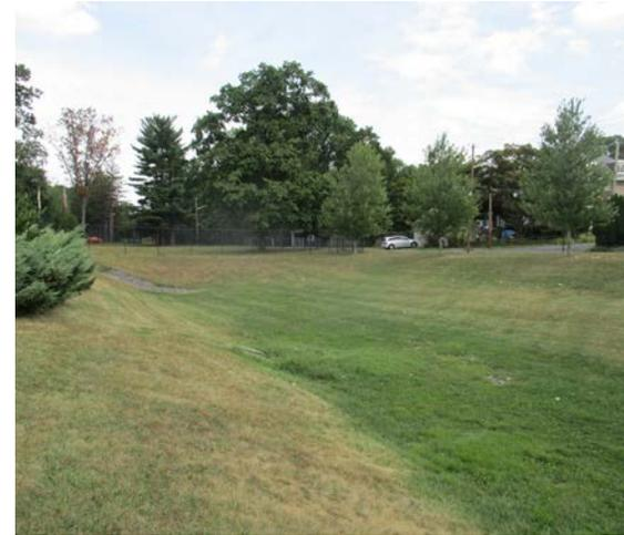
Stormwater is currently draining from west to east across the site. A rain garden can be installed in the adjacent parking island to capture, treat, and infiltrate stormwater runoff from the adjacent parking lot. The nearby stormwater detention basin can be retrofitted to capture, treat, and infiltrate stormwater runoff. A preliminary soil assessment suggests that the soils have suitable drainage characteristics for green infrastructure.
